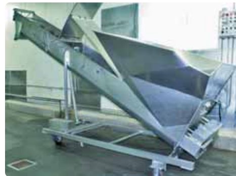
S/S Auger Conveyor
