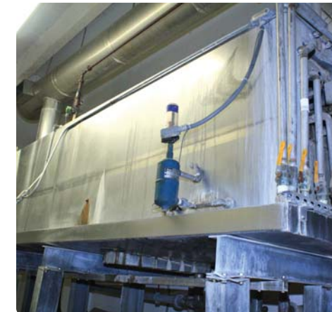
Girton S/S Constructed Case Washer
